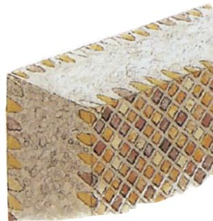
*Antique masonry: Most frequent types of Roman faced concrete building (top to bottom): opus incertum, opus testaceum, and opus reticulatum*
